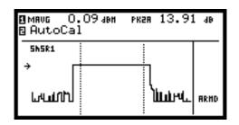
If the power is increased for each pulse, the buffered data array will contain one power reading for each power increment. This can be far faster than recording thousands of data points and analyzing the step increases offline.
